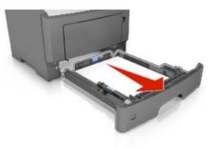
2. Locate the blue lever, and then pull it down to release the jam.
